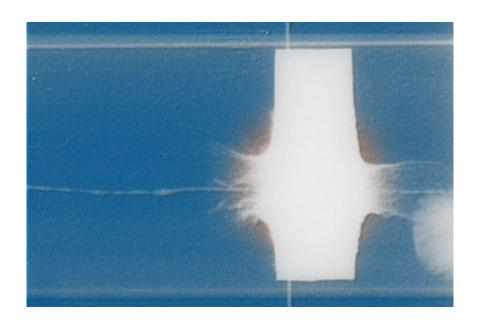
The flash X-ray system can see through smoke and fire to reveal how a projectile or weapon interacts with armor at the exact moment of impact. Here, a copper shape charge, flying from left to right, impacts potential armor material.
