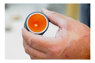
A "shape charge" is a copper lining in the shape of a cone, surrounded on one side with explosive material.
