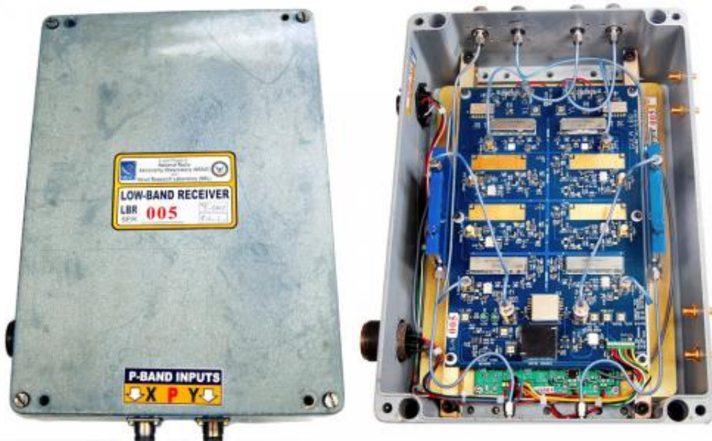
Left: A VLA receiver for the frequency range 50-500 MHz, in its enclosure. These receivers will provide the constant data flow to the VLITE system. Right: Internal view of VLA low-frequency receiver, showing circuit boards and components. Credit: P. Harden, NRAO/AUI/NSF
