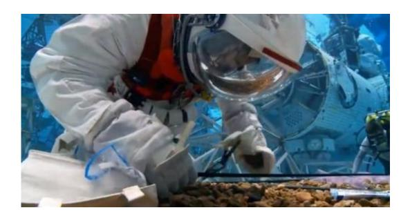
(Phys.org) —NASA is taking steps to make spacewalking on an asteroid a reality. In the Neutral Buoyancy Laboratory (NBL) near the agency's Johnson Space Center in Houston, engineers are testing a modified version of the pumpkin-orange Advanced Crew Escape System (ACES) worn by space shuttle astronauts during launch and reentry for use by future crew in the Orion spacecraft.
