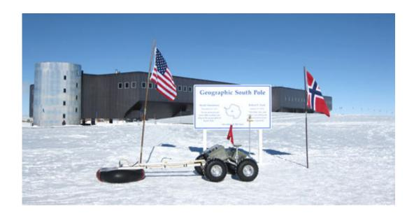
A century after Western explorers first crossed the dangerous landscapes of the Arctic and Antarctic, researchers have successfully deployed a self-guided robot that uses ground-penetrating radar to map deadly crevasses hidden in ice-covered terrains. Deployment of the robot--dubbed Yeti--could make Arctic and Antarctic explorations safer by revealing the potentially dangerous fissures buried beneath ice and snow. Credit: James Lever, U.S. Army's Cold Regions Research and Engineering Laboratory
