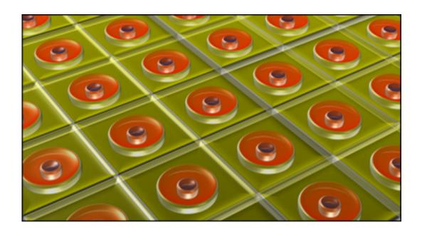
This is a schematic representation of the active layer of the polymer solar cell: The orange dots represent the active domains where light is converted into charge carriers. Credit: Technical University of Munich
