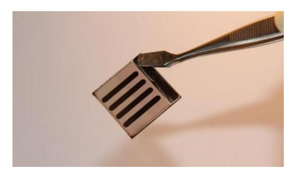
The polymer solar cell sample had an edge length of 10 millimetres. Credit: TU München
