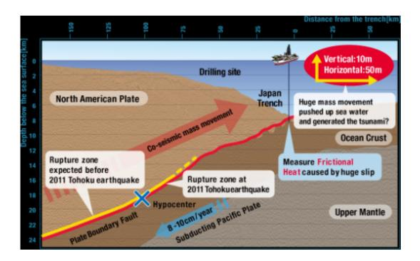
An international team of scientists has concluded that an unusually thin and slippery geological fault where the North American plate rides over the edge of the Pacific plate caused a massive displacement of the seafloor off the coast of Japan in March 2011, touching off the devastating tsunami that struck the Tohoku region. Credit: JAMSTEC/IODP
