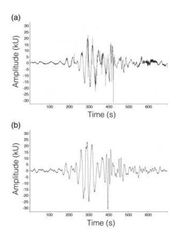
(a) Waveform of a vibration generated by an adult male shuddering in a female's web, and (b) waveform of the same shudder in (a) played through an electromagnetic shaker. Credit: *Scientific Reports* 3, Article number: 3557 doi:10.1038/srep03557
