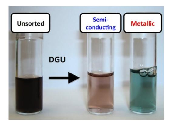
The ability to sort carbon nanotubes by type through a process called "density gradient ultracentrifugation (DGU)" allowed Rice researchers to test purified batches of nanotubes to find the cause of terahertz peaks in spectroscopic experiments. They determined that free electrons formed plasmons that ripple at terahertz frequencies in metallic and doped nanotubes. Credit: Kono Laboratory
