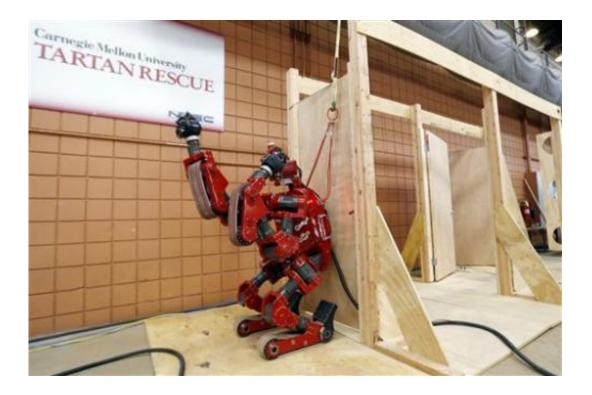
In this photo made on Wednesday, Dec. 11, 2013, the CMU Highly Intelligent Mobile Platform robot, known as CHIMP, finishes a set of doorway tests during a preparation run at the National Robotics Engineering Center in Pittsburgh. Carnegie Mellon researchers are testing the new search-and-rescue robot that
