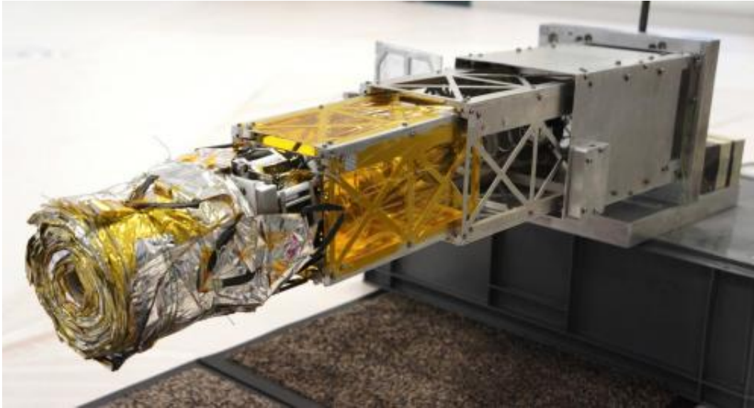
Partially deployed gossamer deorbit sail during testing at the Surrey Space Centre. Credit: University of Surrey
