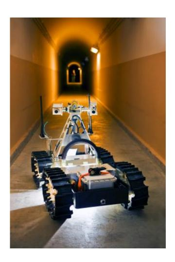
Sandia National Laboratories' Gemini-Scout Mine Rescue Robot is equipped to handle any number of obstacles, including rubble piles and flooded rooms, and to help rescuers reach trapped miners safely and efficiently. Credit: Randy Montoya
