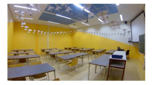
Part of the DelFly Explorer's trajectory during an experiment in a lecture room at TU Delft. The image has been created by copy-pasting the DelFly from different video frames into a single image.
