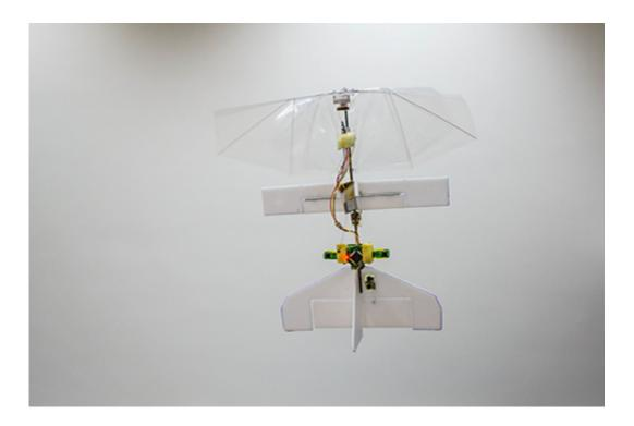
The DelFly in flight with the stereo vision system that allows for autonomous obstacle avoidance.
