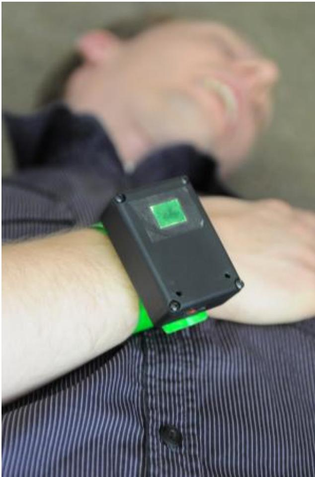
The armband color coding indicates the severity of injury. First responders can decide immediately whether the victim should be taken to a hospital or can be treated on site. Credit: Fraunhofer FIT
