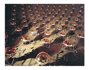
A close-up of the light sensors inside the MiniBooNE neutrino detector. Credit: Fermilab
