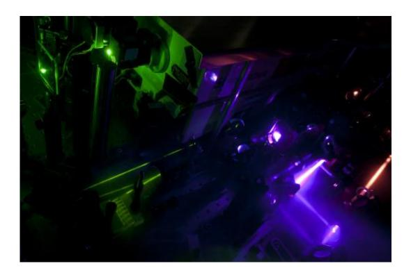
This is the experimental setup used to generate femtosecond laser pulses which serve as an ultrafast "flash" for the camera so that very rapid phenomenon can be filmed. Credit: Simon Gelinas
