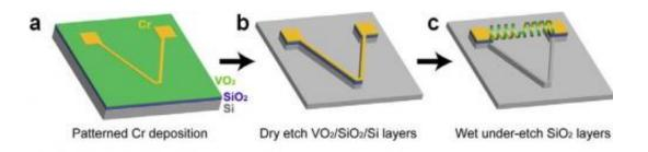
This schematic shows the microfabrication process of a vanadium dioxide-based bimorph dual coil. Credit: Berkeley Lab
