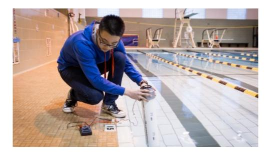
Wake Forest sophomore Yinger "Eagle" Jin ('16) demonstrates his wavepowered electric generator in the pool in Reynolds Gym. The system harnesses the wave action as it compresses air inside the tube, which turns a small turbine that generates electricity.
