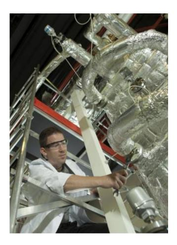
The researchers have also built a heat pump that can raise temperatures to a maximum of 140 degrees Celsius - as opposed to the previous limit of 90 degrees. They use a special process fluid for the heat cycle. The new heat pump makes it possible to boost the temperature of industrial waste heat or heat from geothermal sources from between 70 and 90 to 130 degrees Celsius - the norm in district heating systems. The heat could be used to warm buildings.
