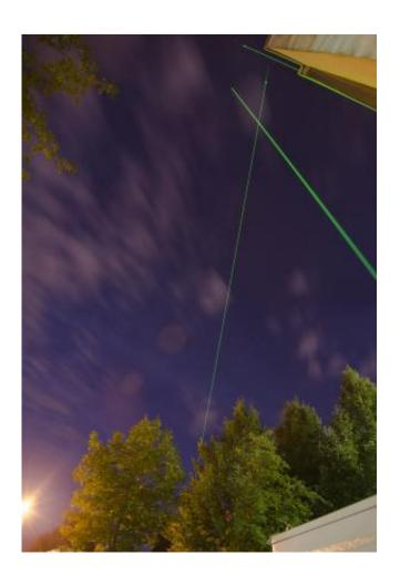
This is the Lidar in use at the TROPOS in Leipzig. With the portable mini-Raman lidar "Polly" a fully automatic system has been developed here, allowing the daily aerosol observations even without much infrastructure. "Polly" has also been used in field experiments in Perl River Delta in China or the Amazon in Brazil. Credit: Tilo Arnhold/TROPOS
