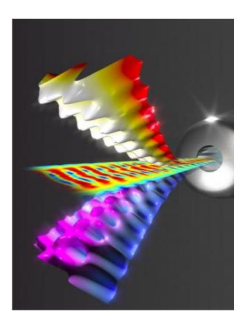
Artist's impression of the experiment. Right: the aluminium needle with fibreoptic core. Left: the middle most plane shows a series of scans above the structure made at different heights, from left (380 nanometres above the crystal) to right (20 nanometres above the crystal). From these measurements the researchers unravelled the electrical (top mountain landscape) and the magnetic (bottom mountain landscape) fields. Credit: Fundamental Research on Matter (FOM)
