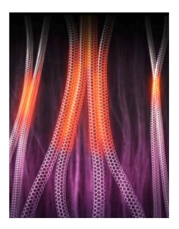
This is a stylized rendition of single walled carbon nanotubes that are just one atom thick in diameter. The red zones show where the attraction caused by van der Waals forces has bent or "zipped" two adjacent CNTs together. Credit: Alex Jerez.
