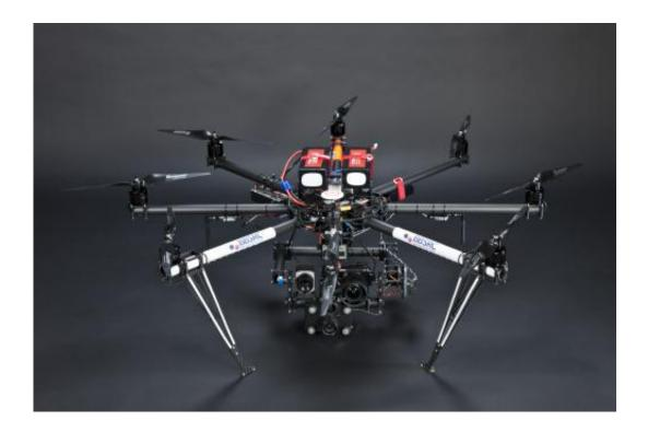
The octocopter is a standard 8 rotor battery powered unmanned aerial vehicle, as typically used in the film industry. Four cameras have been added, two of which at any time can give a live feed of their picture to a monitor on the ground. Credit: Rothamsted Research
