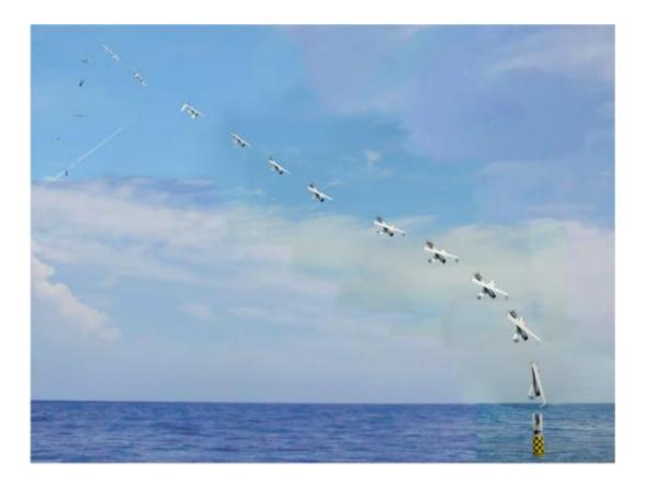
XFC UAS launch in time-lapsed photography. Deployed from the submerged submarine USS Providence, the NRL developed XFC unmanned aircraft is vertically launched from a 'Sea Robin' launch vehicle (bottom right). The folding wing UAS autonomously deploys its X-wing airfoil and after achieving a marginal altitude, assumes horizontal flight configuration. Credit: (NAVSEA-AUTEC)
