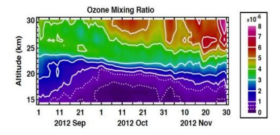
A look inside the 2012 ozone hole with the Ozone Mapper and Profiler Suite shows how the build-up of ozone (parts per million by volume) in the middle stratosphere masks the ozone loss in the lower stratosphere. Credit: NASA
