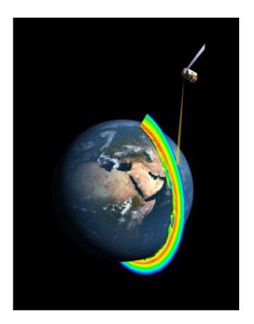
This is a cross-section of Earth's ozone layer as measured by the limb profiler, part of the Ozone Mapper Profiler Suite that's aboard the Suomi NPP satellite. Credit: NASA/NOAA
