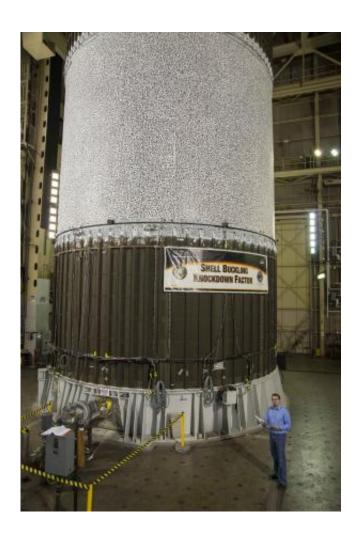
NASA's Mark Hilburger prepares to buckle an aluminum-lithium cylinder about the size of fuel tank barrels for the largest rockets ever built. The black and white dots on the upper portion of the tank helped 20 high-speed cameras record minute changes in the tank as almost a million pounds of force pressed down upon the tank in a test at NASA's Marshall Space Flight Center.
