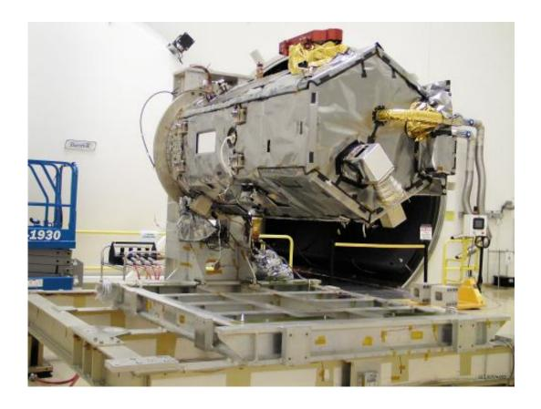
NASA's Orbiting Carbon Observatory (OCO)-2 spacecraft sits "on its back" atop ground support equipment at Orbital Sciences Corporation's Satellite Manufacturing Facility in Gilbert, Ariz., in preparation for environmental testing. The observatory's solar array panels were removed prior to the test. Image credit: Orbital Sciences Corporation/NASA/JPL-Caltech
