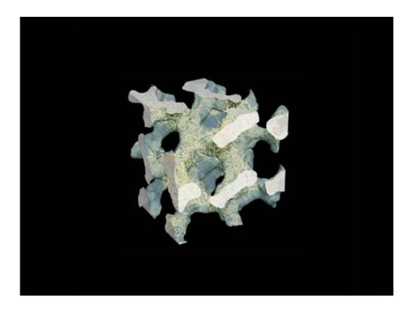
A schematic view of a mesoporous polymer. Polymer assemblies in nanofiber form with pores of 10 to 20 nm in diameter are branched in a sophisticated fashion to create a minute three-dimensional network structure. The yellow lines represent assemblies of polymer chains that form nanofibers.
