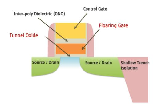
Fig.1 FLOTOX Structure
