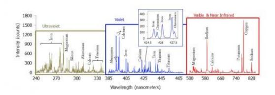
The averaged spectrum of point 1 from the target "Ithaca", which includes data from the 100,000th laser shot by ChemCam. This spectrum is typical of Martian volcanic (basaltic) material, from which the sediments in Gale are derived, with a standard major element suite of Si, Mg, Al, Ca, Na, K, O, and Ti. There is an enrichment in Fe (>20% FeO) and Ti (>1% TiO2). Chromium and Mn (not shown) are also present. Credit: Los Alamos National Laboratory
