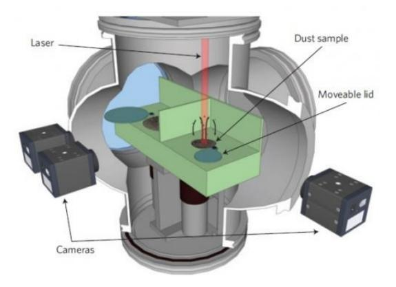
Schematic diagram of the drop tower experiment. Basaltic dust is illuminated with a red laser as the entire device falls from the drop tower in Bremen, Germany. Credit: de Beule, et al. ©2013 Macmillan Publishers Limited. All rights reserved.
