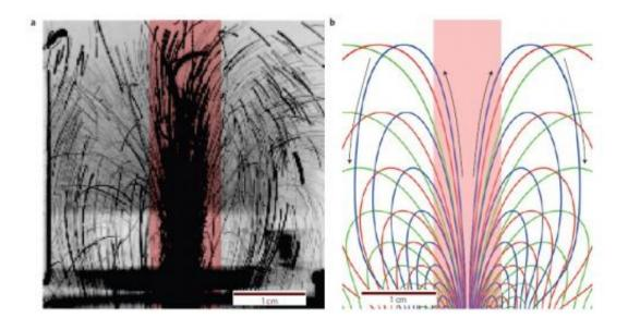
Particles trajectories (a) in experiments above an illuminated dust bed are consistent with those (b) in gas flow simulations. In both cases, gas quickly flows upward in the center illuminated (red) area, and falls downward more slowly on the sides. Credit: de Beule, et al. ©2013 Macmillan Publishers Limited. All rights reserved.
