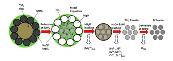
A novel method for extracting titanium, a metal highly valued for its light weight, high strength, corrosion resistance and biocompatibility, could lower its cost and make it more widely accessible, for example, for producing lighter car parts to improve fuel efficiency. The method, which significantly reduces the energy required to separate it from its tightly bound companion, oxygen, appears in the *Journal of the American Chemical Society*.
