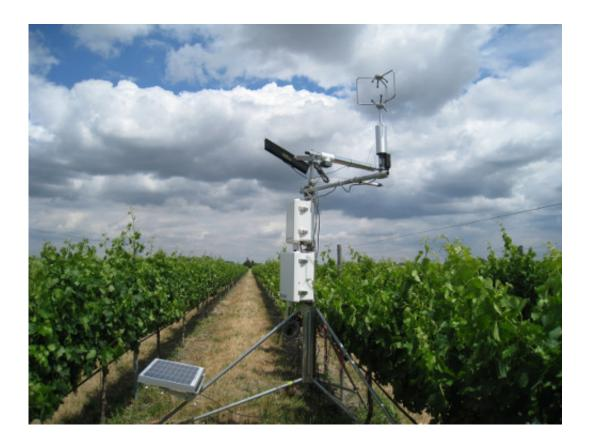
This is a solar powered field station established in a vineyard in California to measure surface renewal. Credit: *JoVE*, the *Journal of Visualized Experiments*
