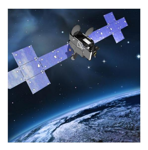
This is an artist rendering of the Laser Communications Relay Demonstration hosted aboard a Space Systems Loral commercial communications satellite. Credit: Space Systems/Loral
