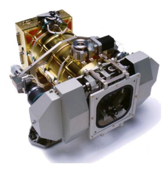
This is the Total Irradiance Monitor used to measure solar irradiance on the TCTE and SORCE missions. Credit: LASP, University of Colorado
