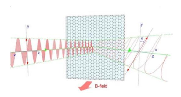
Phase and amplitude modulation of light by a single sheet of graphene. Credit: (US Naval Research Laboratory)
