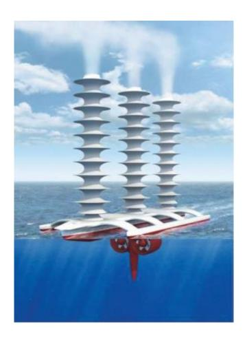
A conceptualized image of a wind-powered, remotely controlled ship that could seed clouds over the ocean to deflect sunlight. Credit: John MacNeill
