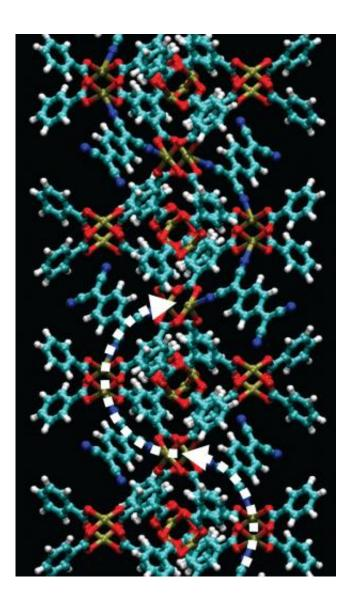
Electron-sharing TCNQ molecules bind to the copper ions in the framework to enable electrical conductivity in MOF materials. The dotted white arrows
