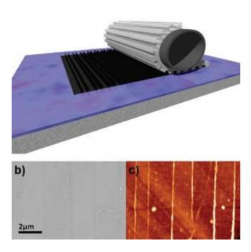
(a) To grow graphene fin-like structures, the researchers draped a graphene sheet over a patterned stamp. Below, (b) a scanning electron micrograph and (c) an atomic force microscope image show a small portion of the folded graphene surface. Credit: A. T. Costa, et al. ©2013 EPL
