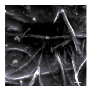
Graphene nanoribbons embedded in polyurethane paint, seen in an electron microscope image, are part of a deicing solution created by Rice and Lockheed Martin. The scale bar equals 1 micrometer. Credit: The Tour Group
