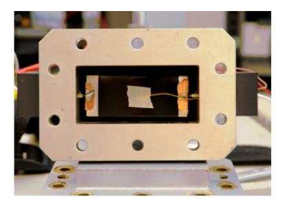
A waveguide in the Rice University lab of chemist James Tour frames a graphene nanoribbon film for testing. Rice developed the material as a thin, robust deicer for radar domes and other applications.Credit: Tour Group
