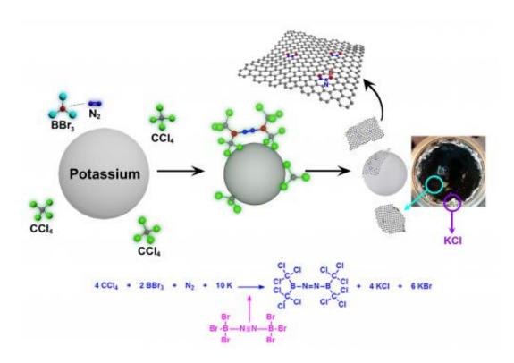
This is a schematic representation for the formation of BCN-graphene via solvothermal reaction between carbon tetrachloride (CCl4) boron tribromide (BBr3) and nitrogen (N2) in the presence of potassium (K). Photograph is of the autoclave after the reaction, showing the formation of BCN-graphene (black) and potassium halide (KCl and KBr, white). Credit: UNIST
