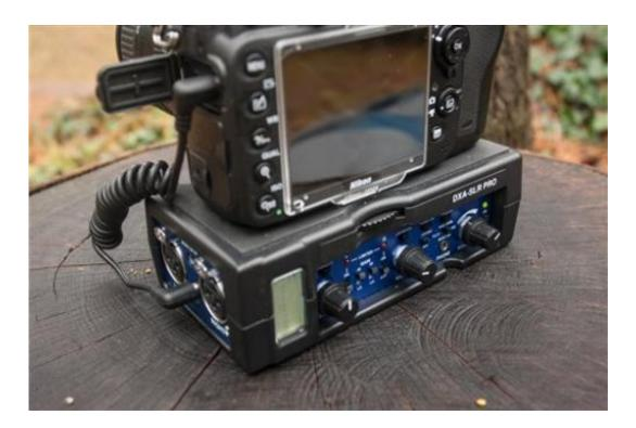
The Beachtek DXA-SLR PRO audio adapter is shown on Tuesday, Dec. 3, 2013 in Decatur, Ga. The device can be mounted to the bottom of a DSLR camera and provide professional audio mixing capabilities to the sounding recording of the video footage. (AP Photo/ Ron Harris)
