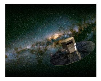
Gaia weighs 2,100 kg, it is 3.5 meter high and has a diameter of 10 meters. The instruments are placed on a hexagonal optical bench. At the bottom are solar panels that supply the satellite with 2,000 watts of power. Credit: ESA
