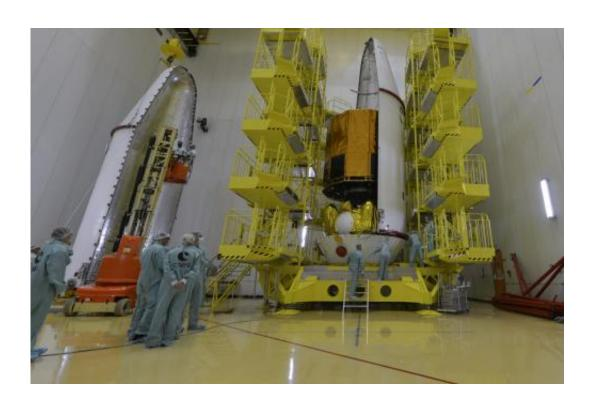
The Gaia spacecraft is positioned inside the Soyuz fairing, in preparation for the 19 December 2013 launch. The spacecraft was attached to the vehicle adapter before being installed in the fairing. Launch is scheduled for 9:12:19 GMT (10:12:19 CET) on 19 December 2013. Credit: ESA–M. Pedoussaut
