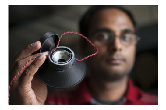
Graduate student Apoorva Kiran holds a 3-D printed, fully functional loudspeaker. Credit: Jason Koski/University Photography
