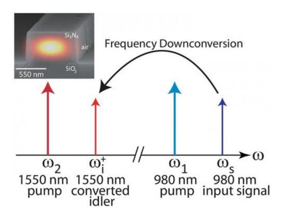
s shown in the schematic, in frequency downconversion, an input signal at 980 nm is frequency shifted to the 1550 nm wavelength band through the application of two strong pump lasers. The reverse process of upconversion (shifting an input signal from 1550 nm to 980 nm) was also demonstrated. Inset: Scanning electron micrograph of the cross-section of a silicon nitride waveguide designed for the frequency conversion with a simulation of the device's optical field profile superimposed.
