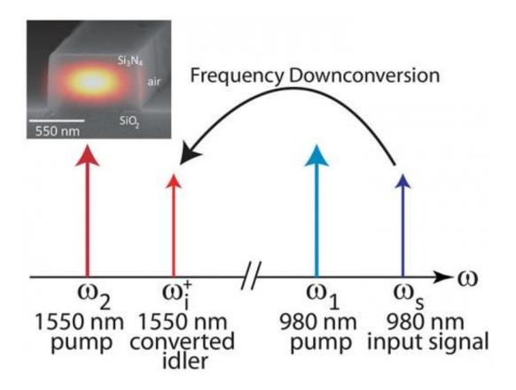
s shown in the schematic, in frequency downconversion, an input signal at 980 nm is frequency shifted to the 1550 nm wavelength band through the application of two strong pump lasers. The reverse process of upconversion (shifting an input signal from 1550 nm to 980 nm) was also demonstrated. Inset: Scanning electron micrograph of the cross-section of a silicon nitride waveguide designed for the frequency conversion with a simulation of the device's optical field profile superimposed.
