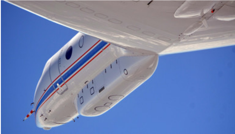
Fig. 2: "Belly Pod" underneath the hull of HALO. It contains radiometers, a radar and a laser for measuring profiles during the flights. Credit: DLR
