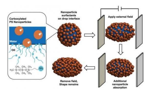
Schematic shows how the application of an electrical field transforms a spherical drop clad with nanoparticle surfactants into an ellipsoid.
