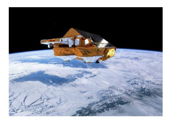
ESA's Earth Explorer CryoSat mission is dedicated to precise monitoring of changes in the thickness of marine ice floating in the polar oceans and variations in the thickness of the vast ice sheets that blanket Greenland and Antarctica. Credit: ESA/AOES Medialab
