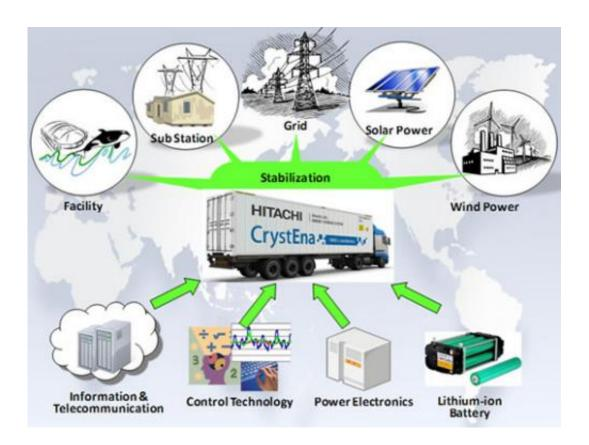
Hitachi today announced that it has developed an all-in one, containertype energy storage system as a core energy product for ensuring the stable use of distributed renewable energy such as wind and solar power, while maintaining the power supply-demand balance. This energy storage system fuses Hitachi's electricity grid control technologies built
