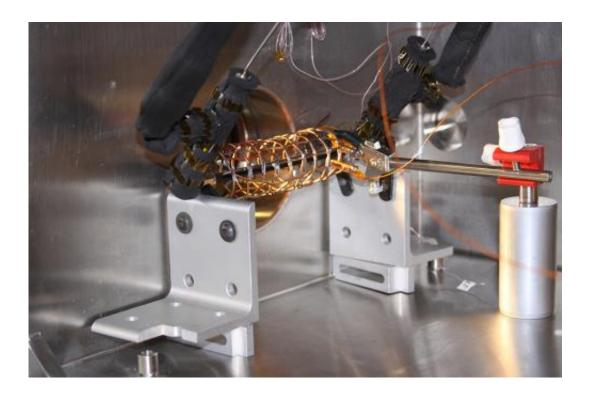
An open structure of copper wire surrounding a pipe was used in the lab to measure how effective an electric field can be in pulling droplets away from a condenser surface. In combination with a particular kind of superhydrophobic surface, the new system can nearly double the efficiency of the cooling process, the researchers found.
